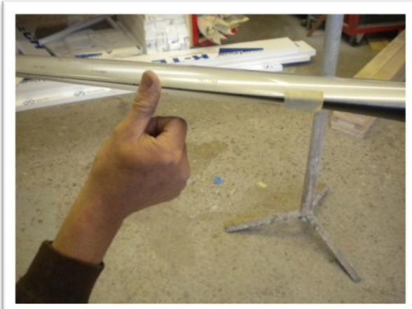
the tape about a half inch. As you do this the tape around the tip will begin to fold around and over the blade tip curvature.
