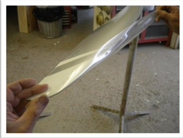
Starting at about  $1/3^{\text{rd}}$  the way around the tip radius, apply just the very edge of the LET with the majority of the adhesion being on the masking tape at the tip. It is important not to go further than the  $1/3^{\text{rd}}$  way around the tip, otherwise you will get excessive wrinkling of the tape.
