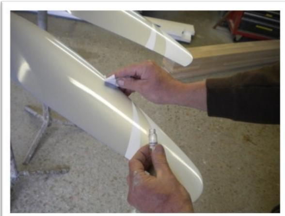
Make sure the propeller is clean and free of any grease or contaminants. You can use Windex or any type of wax and grease remover. Apply a generous amount of the LET Adhesive Enhancer supplied to the leading edge area the tape will be bonded to. Use a small piece of paper towel or similar to apply. This will usually take about 15 minutes to dry.
