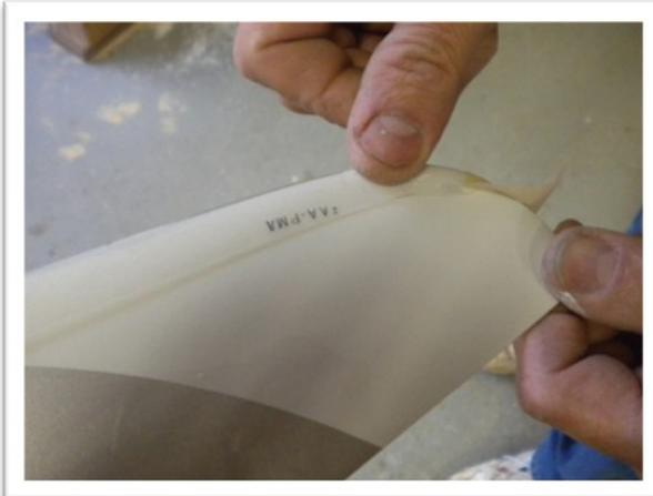
The tip region and radius is the most tedious area to do. Depending on how far you stretched the LET when you applied it will depend on how many and how bad the wrinkles are at the tip radius. Working from the leading edge aft, work the tape back and forth and even out any wrinkles as you go.
